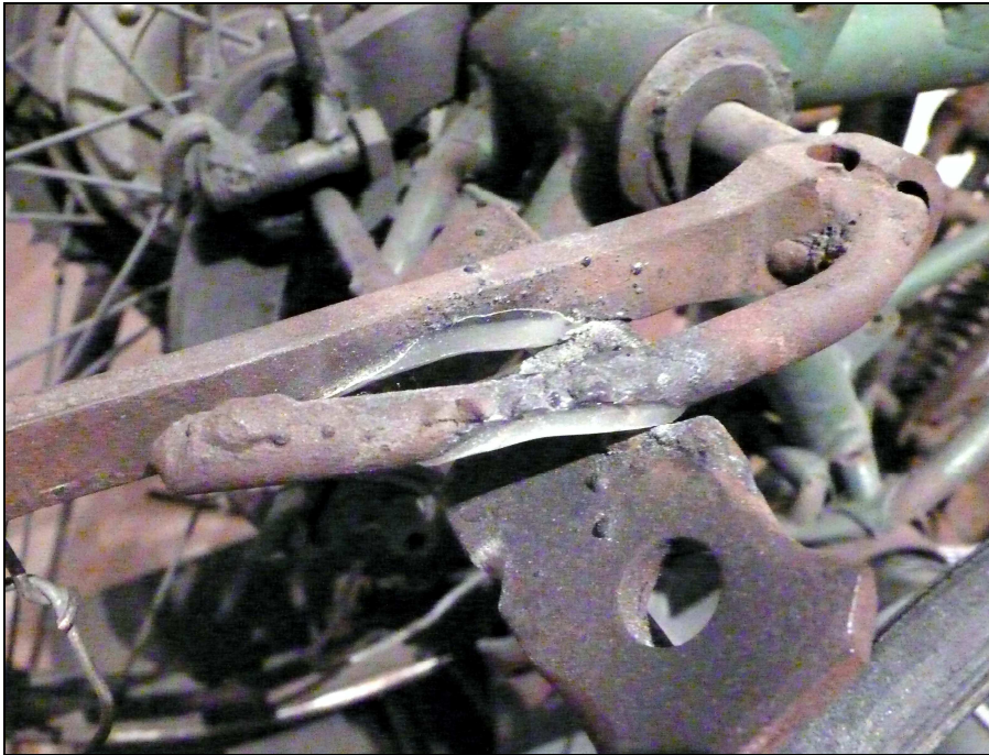
Fig. 1: Wear Layer of Epoxy Resin on a Pedal with High Friction after Two Years on Exhibition
