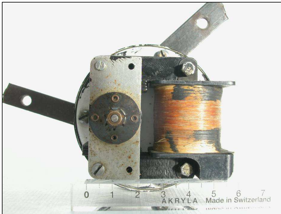
Fig. 35. Back of motor. Left: the round rotor, surrounded by the iron core. Right: iron core surrounded by the main winding.
