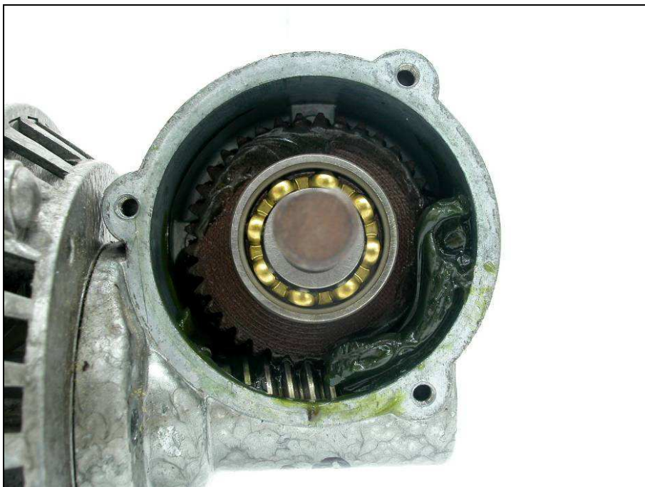
Fig. 30. View into the gearbox showing gear of fiber-reinforced plastic.
