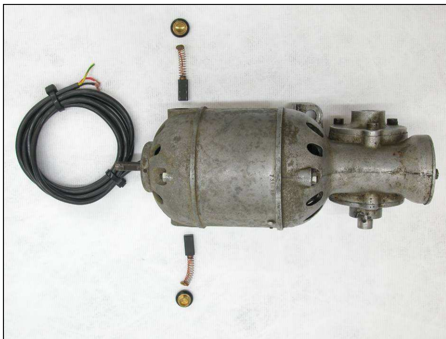
Fig. 6. Disassembled carbon brushes
