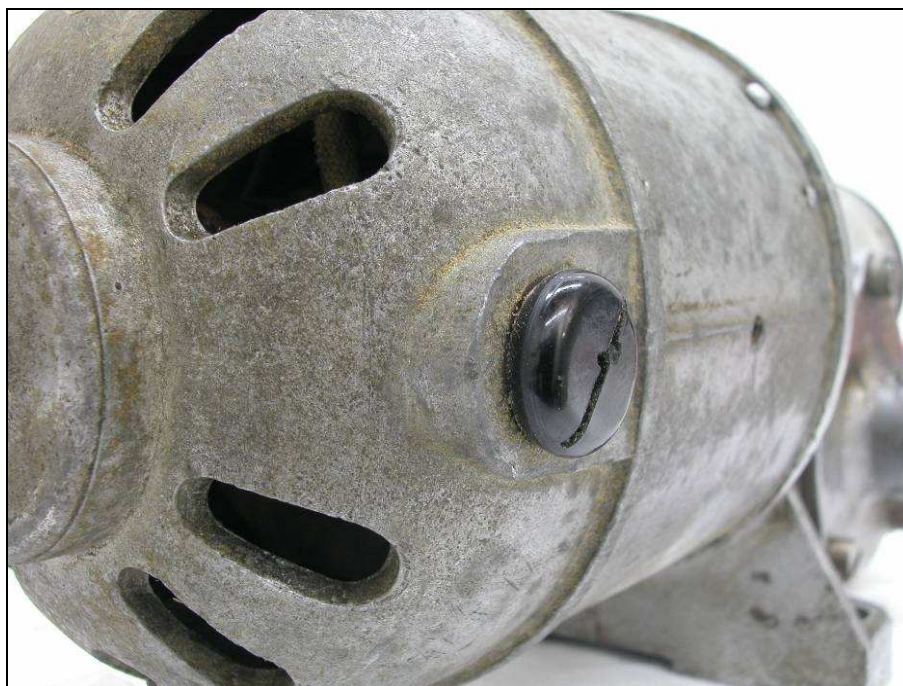
Fig. 4. Screw cap to secure carbon brushes
