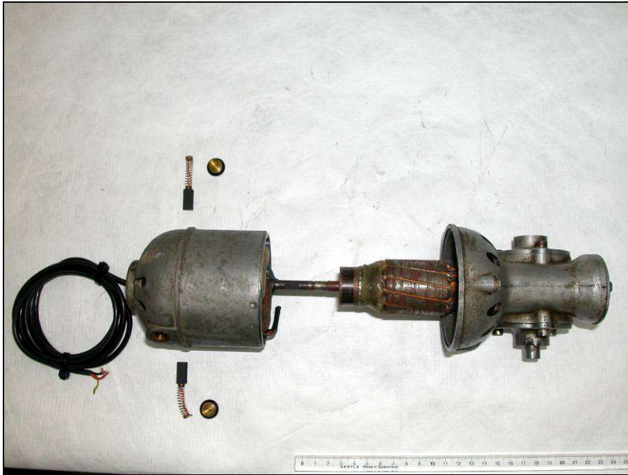
Fig. 7. Disassembled motor housing with exposed armature shaft
