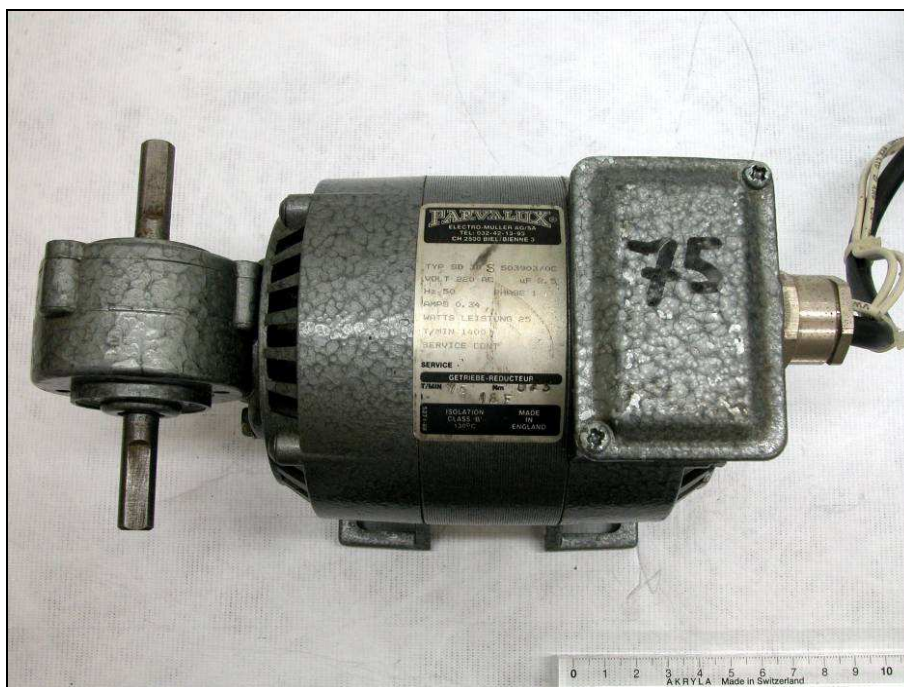
Fig. 18. View from above showing cover of terminal box.
