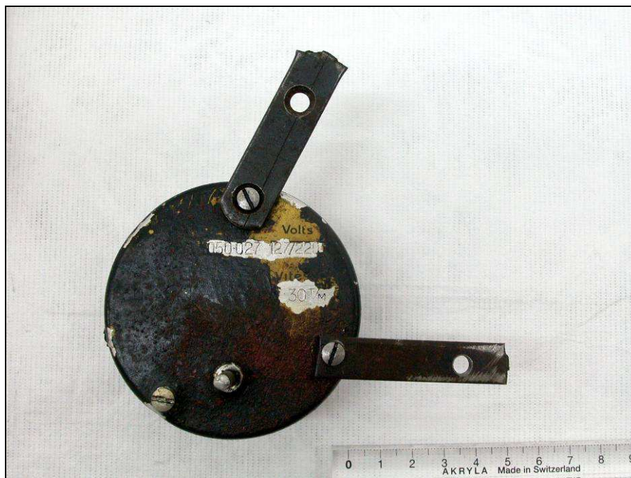
Fig. 32. Shaded-pole motor by SAPMI
