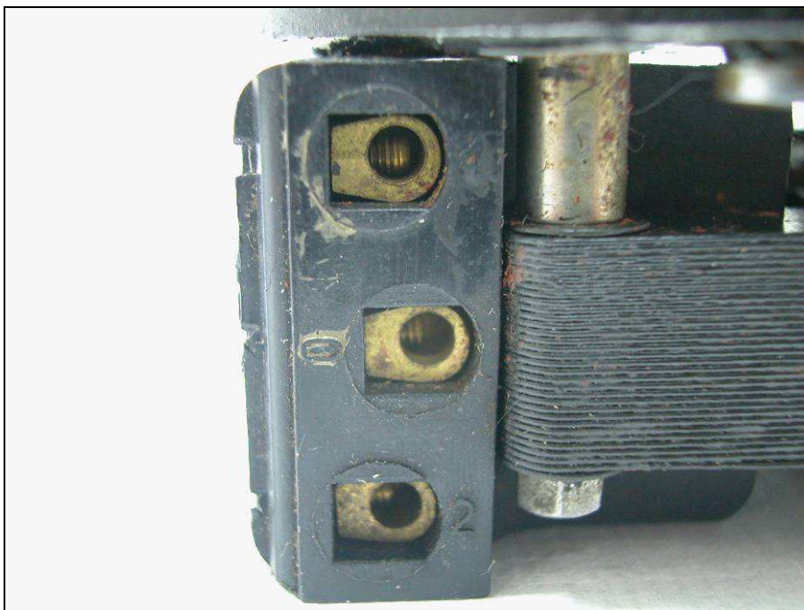
Fig. 36. Terminals: 0 and 1 for 127 volts / 0 and 2 for 220 volts
