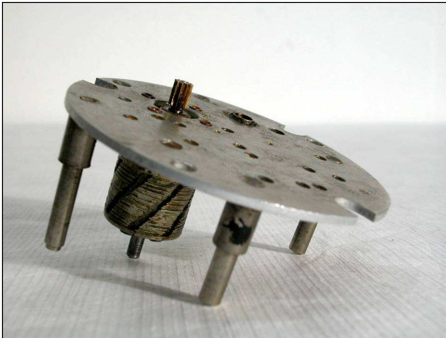
Fig. 42. Base plate with squirrel-cage rotor and its drive gear.
