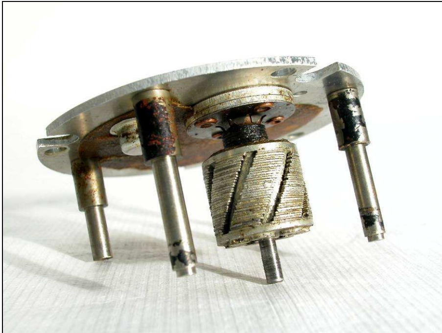
Fig. 43. Base plate with squirrel-cage rotor.
