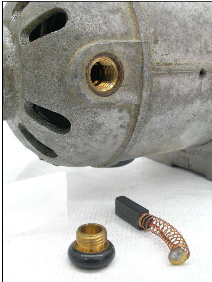
Fig. 5. Disassembled carbon brush with pressure spring
