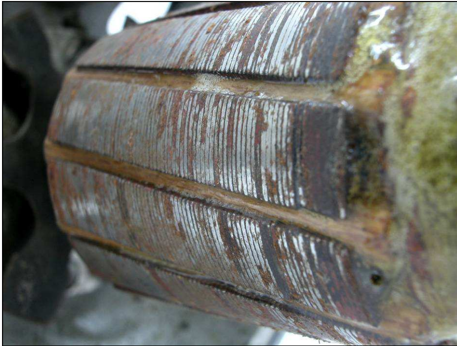
Fig. 13. Rotor with slots in the sheet metal of the armature. The surfaces are corroded.
