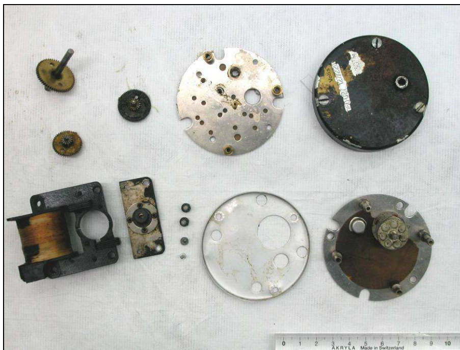
Fig. 46. All the components of a shaded-pole motor
