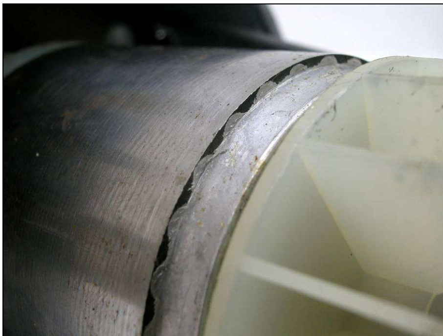
Fig. 28. Detail of rotor: The rotor coils are squirrel-cage conductive loops.
