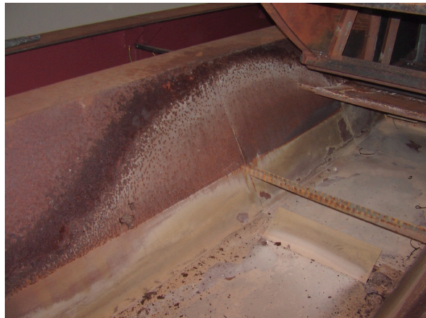
Fig. 7: as fig. 6 after 24 months of presentation: considerable augmentation of corrosion. (October 2006) (photo: ZKM)
