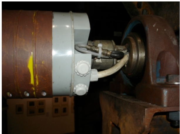
Fig. 13: Original slip ring unit and its connection to the wheel axle (August 2004) (photo: ZKM)
