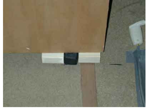
4. The right back wheel of the box, the wooden guide strip and the position mark
