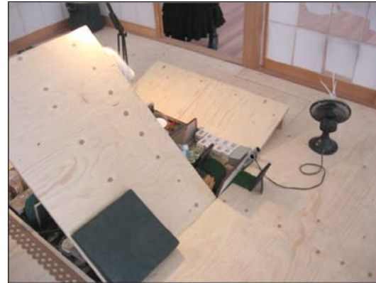
The fan is on and is blowing in the direction of the loose sheets in the panel.
