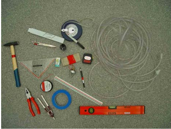
Fig 21: Equipment used for hand measurement taking account of deformations.
