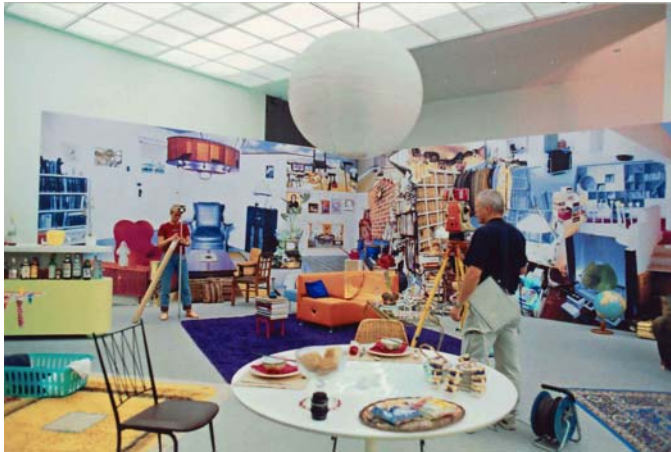
Fig. 11: Tachymetric measurement of the key points. Here, one of the corners of the carpet.
