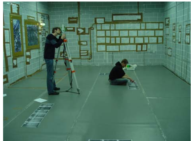
Fig. 38: Tachymetric measurement for the photogrammetric equalisation of the images.
