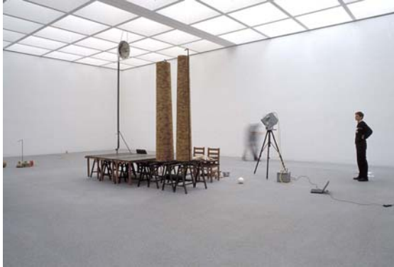
Fig. 29: The laser scanner, here on a tripod, was set up in ten different positions around the artwork.
