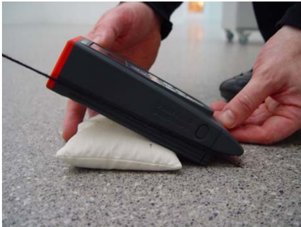
Fig. 18: The sand bag serves to stabilize the focusing of the range finder parallel to the cord.
