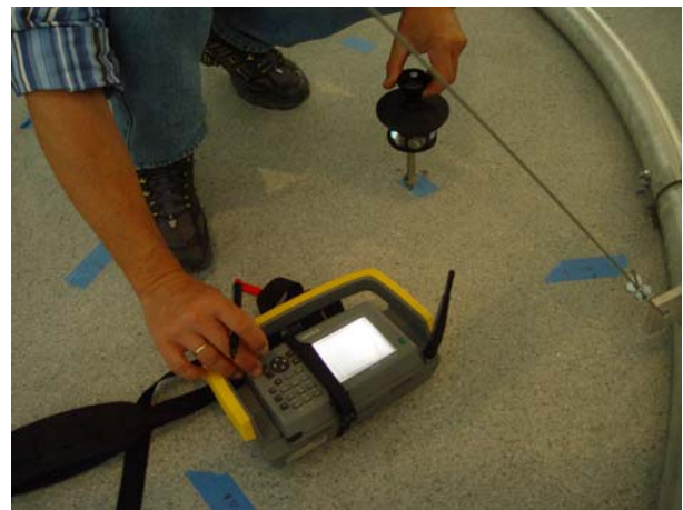
Fig. 46: Tachymetric measurement of the measuring points on the colour lengths.
