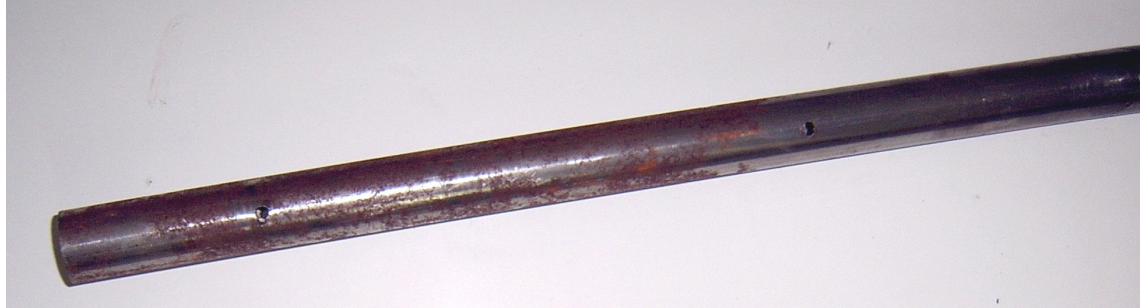
Rust on the end of the bar.
