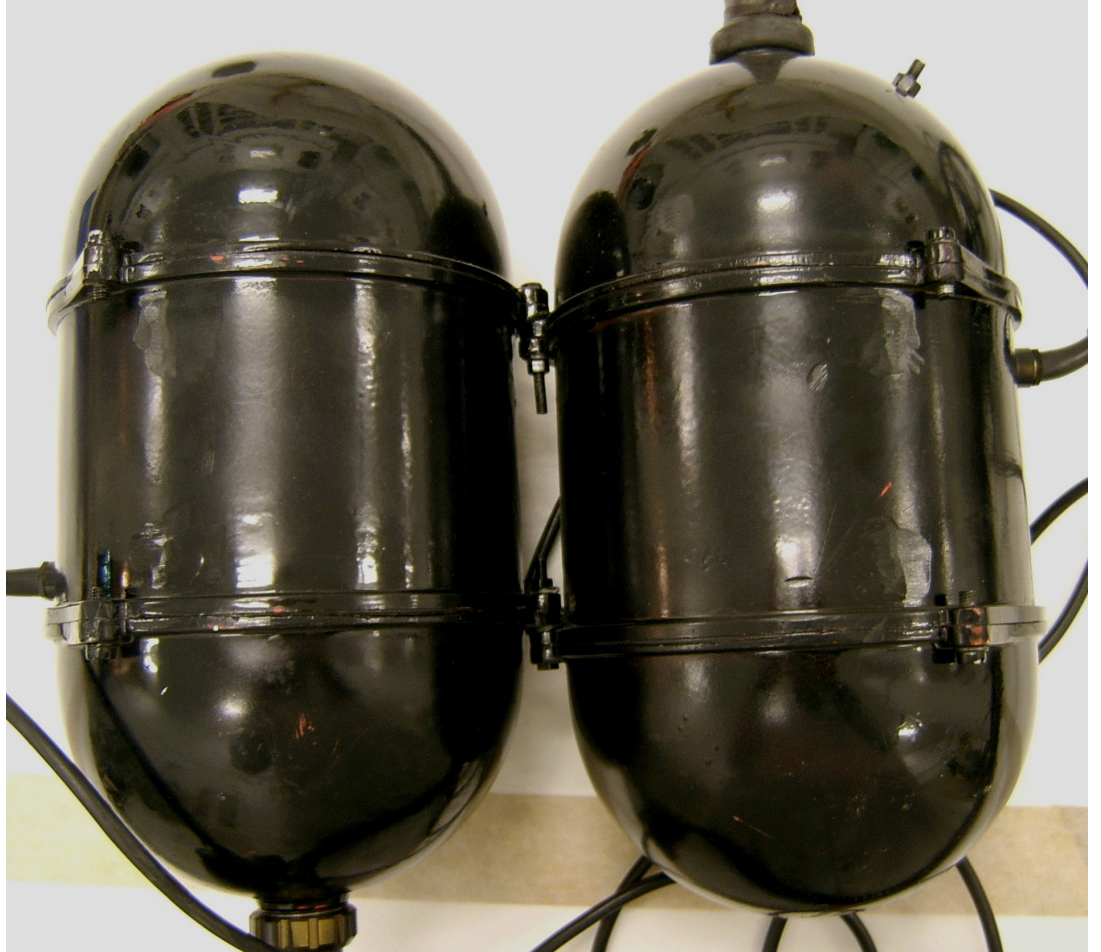
Scratches and bald patches in the paint on the compressor.
