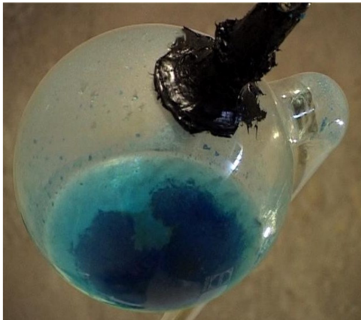
State of the copper sulphate. 2/3 of the water has evaporated, leaving residues of blue and black sulphate.
