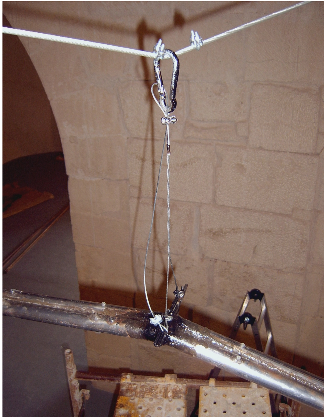
View of the central axis attached to the cable. This axis is twisted several times so that it will rotate anticlockwise.
