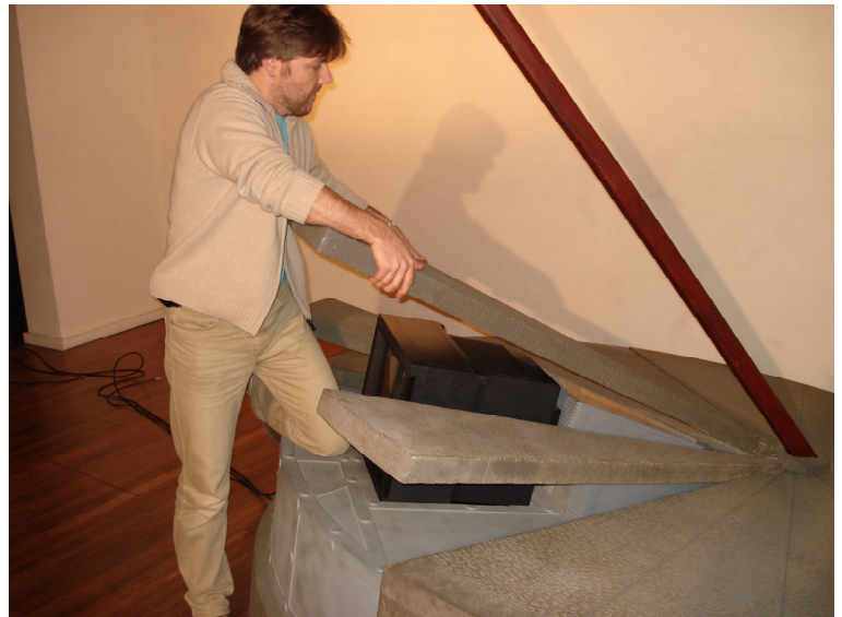
15. Place the monitor cover (Part I) onto part G and the monitor (part H)
