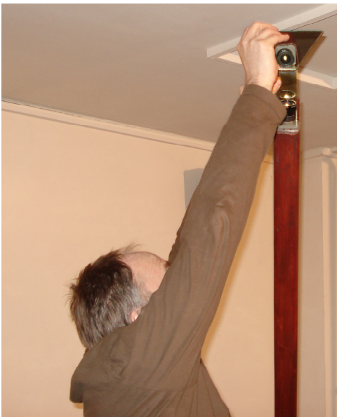
13. Adjust mirror on top of camera to get the desired angle (a person in front of AA should be seen entirely on the screen when standing approx. 1.5 to 2m away from AA).
